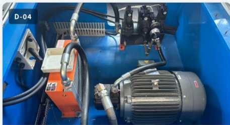
Hydraulic Power Unit HYDRAULIC UNIT Taiwan motor with CML solenoid valve bank, oil cooler and Japan NOK seals — tidy piping and stable power.
