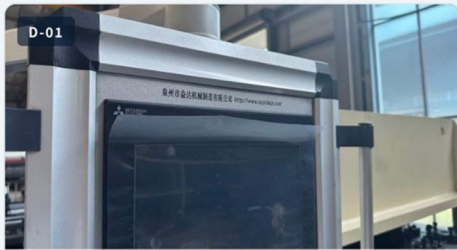
Mitsubishi 10" Touchscreen MITSUBISHI HMI Large color touchscreen with intelligent menu — one-touch parameter setting and real-time display.
