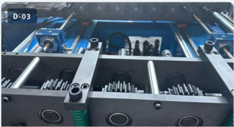
Precision Drive System DRIVE SYSTEM Worm-gear reducers with cross ball screw and guide shafts, paired with HIWIN linear guides for precise width adjustment.
