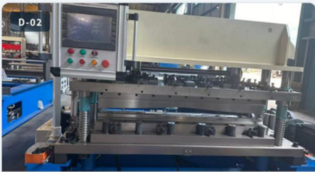
Operation Panel CONTROL PANEL Power/device indicators, start, pause, alarm reset and E-stop arranged clearly for safe, convenient operation.
